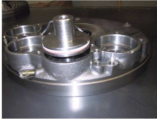
FIGURE 80 EMMA piston installation
