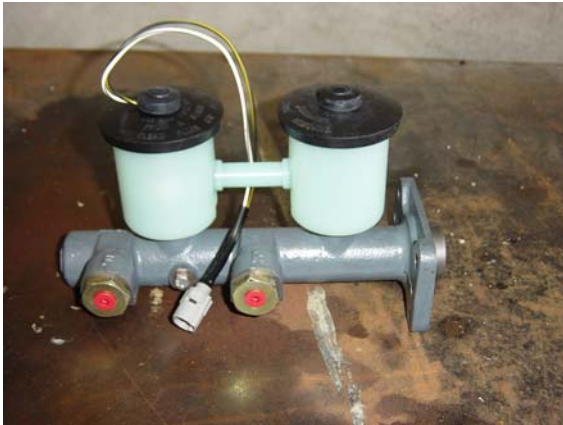
New master cylinder. Note level switch and connection between reservoirs
