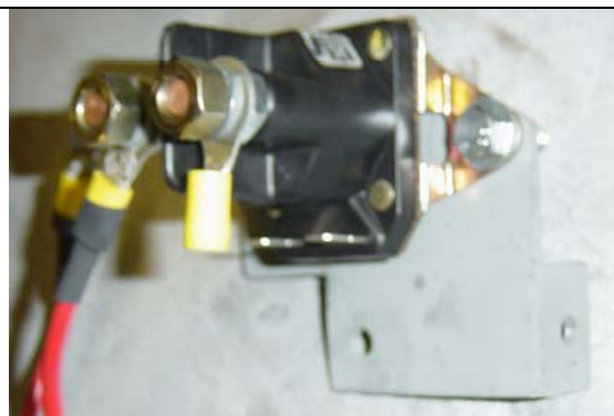
Relay shown fixed to a bolt-on bracket. Supplied bracket can be bolted to existing bracket via
