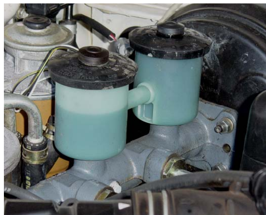
Previously supplied 1” bore master cylinder with SIBS rear only kits.
