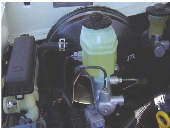
Standard Toyota master cylinder in 70 series Landcruiser. Bore: 15/16”.
