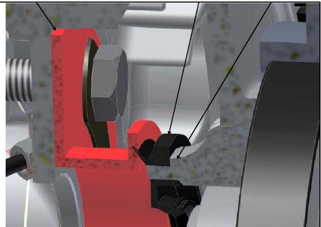
Close up showing seal carrier (red), v-seal and SIBS wheel bearing seal.
