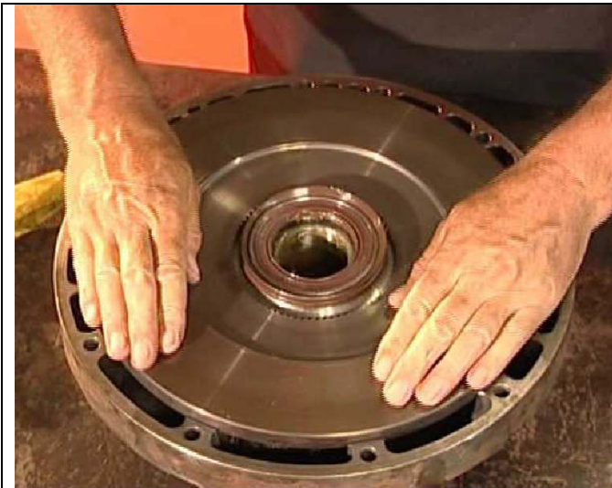
Figure 7 Preparing outer housing / hub / rotor / pad assembly for fitment to inner housing. Place outer housing over hub. Install pads and rotor.
