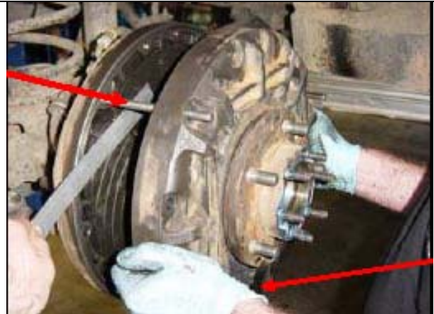
Figure 4 Remove outer housing / hub / rotor and outer pads as one assembly. Have a colleague hold the inner pads with a steel rule to prevent them falling on the ground.
