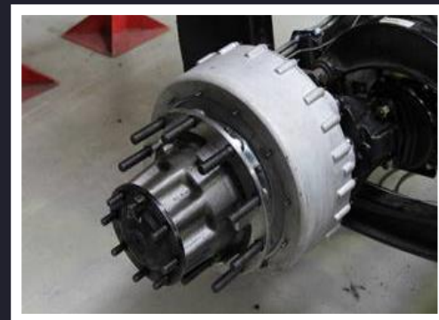
Diagram 2: Truck brake installed on rear axle of a Iveco ACCO truck
