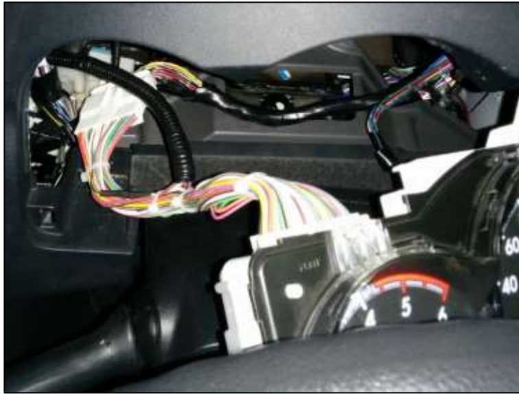
Figure 32: Connect the vehicle interface harness between the instrument cluster and 40-pin white OEM plug.
