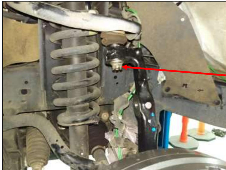
Figure 15: Install suspension upper arm.
