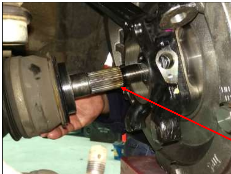
Figure 16: Slide axle into housing.
