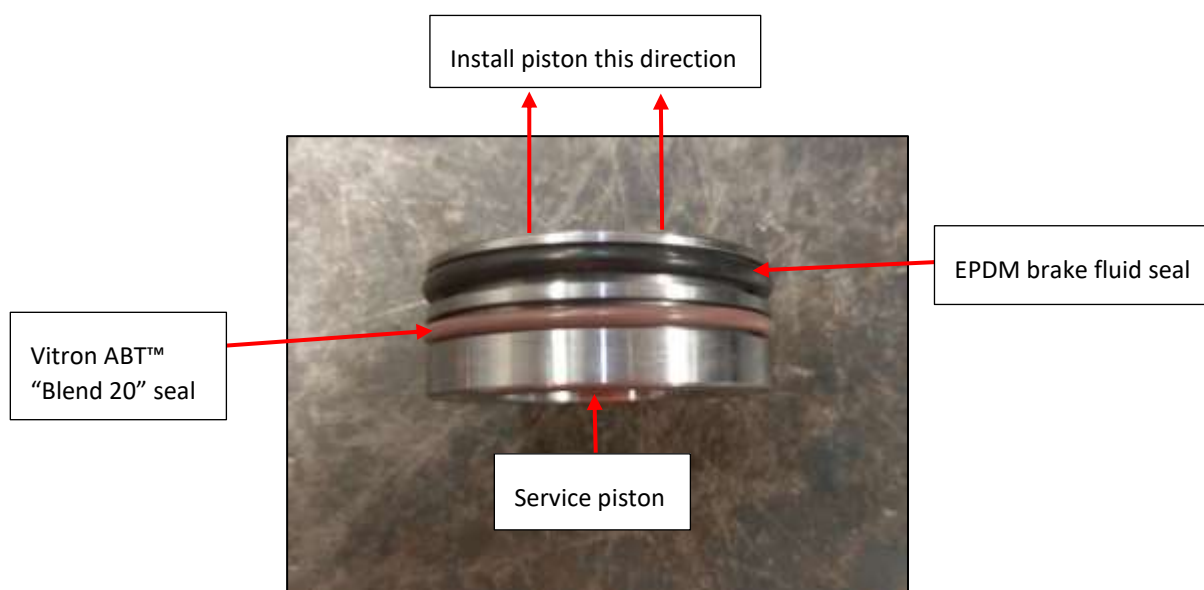
Figure 57: Piston O-ring positions
