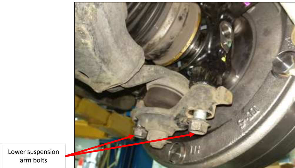
Figure 17: Install suspension low arm.
