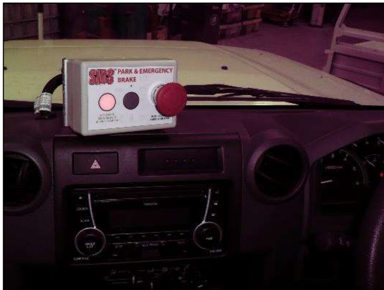
Figure 29: ABT™ Failsafe control unit mounted on dash.
