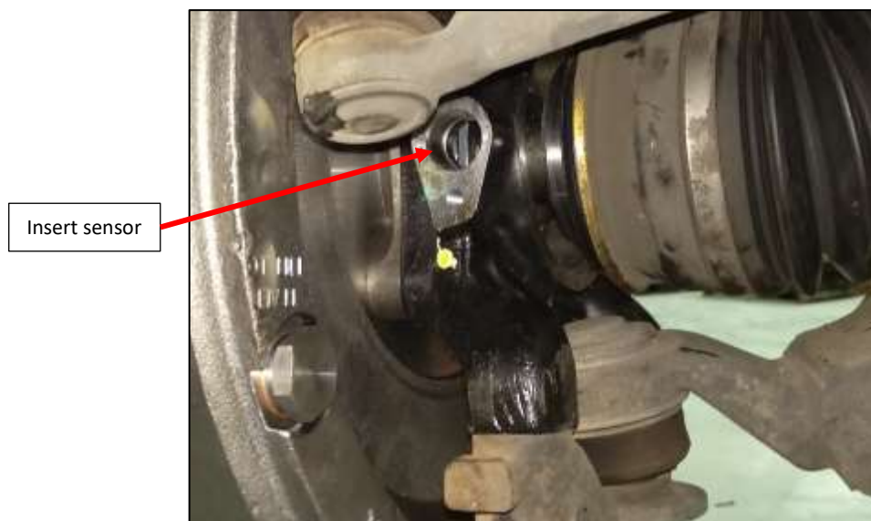
Figure 22: Install ABS sensor.
