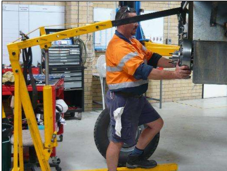
Figure 5: Carefully fit brake assembly over stub axle.
