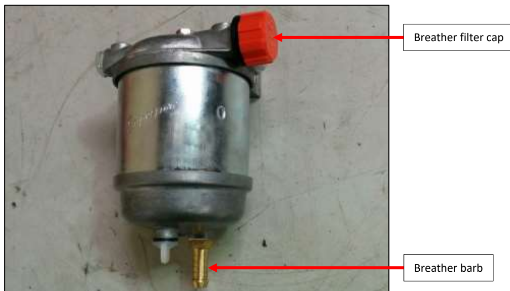
Figure 24: Mount the expansion chamber in the engine bay.
