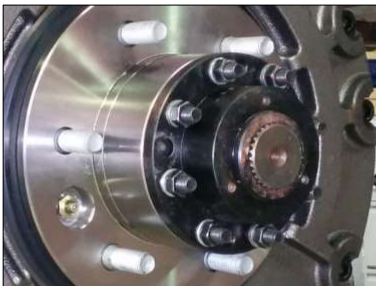
Figure 8: Fit the axle drive flange.
