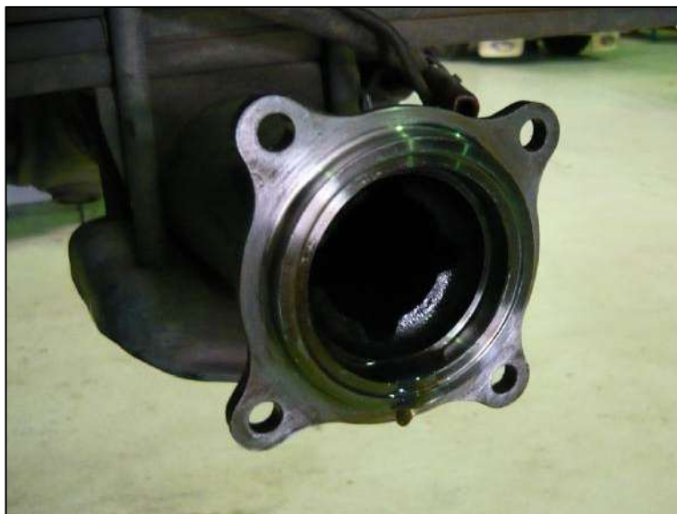
Figure 1: Prepare axle flange.
