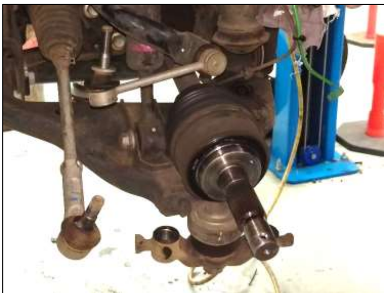
Figure 13: Remove OEM front brake equipment.
