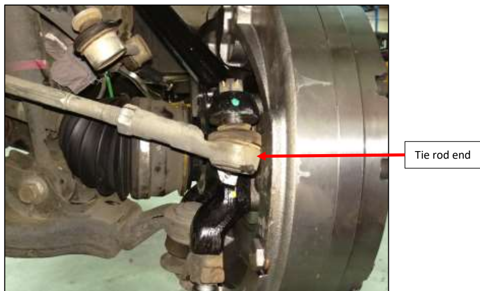
Figure 18: Install tie rod end.
