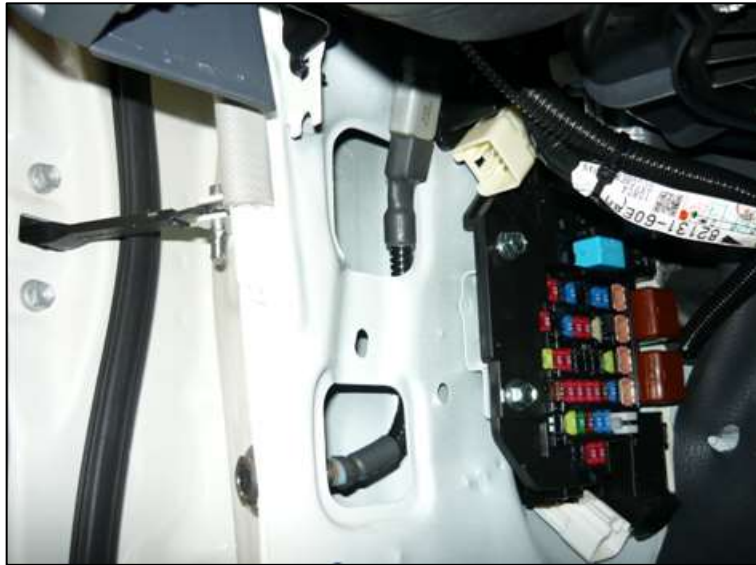
Figure 35: Secure proximity switch with locknuts and route harness.
