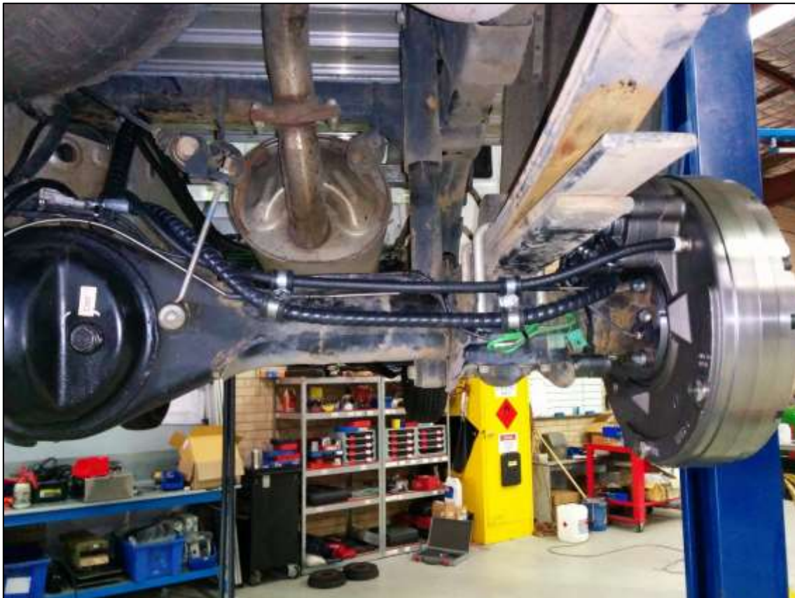
Figure 27: Brake lines routed to rear RH brake unit (facing front of vehicle).
