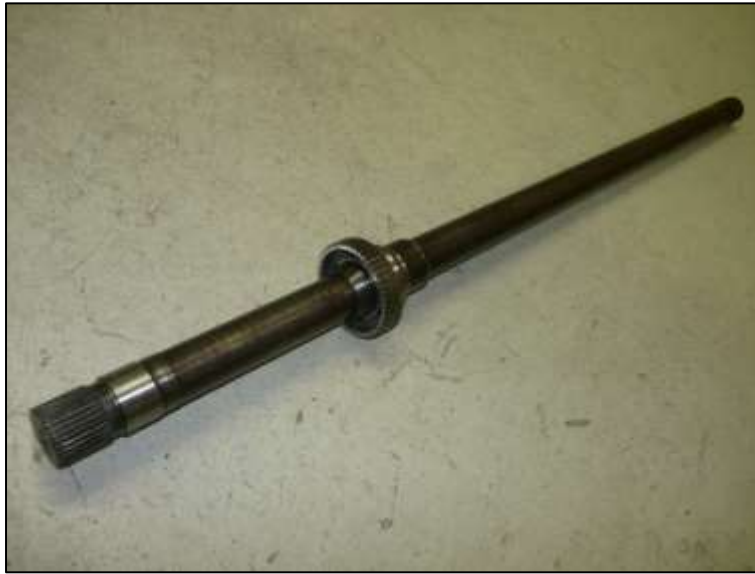
Figure 3: Fit ABS pulse wheel to axle.
