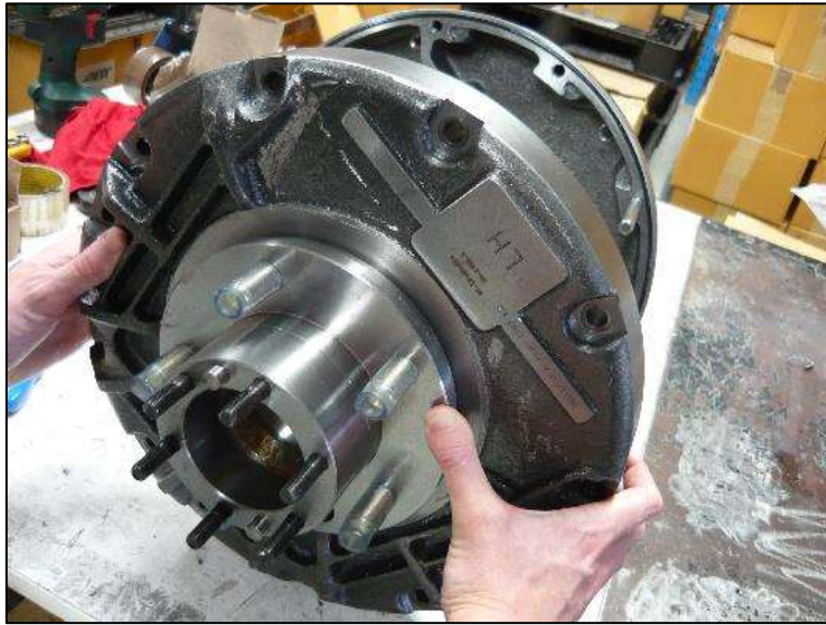
Figure 43: Separate inner and outer housings.
