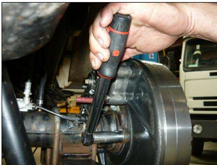
Figure 6: Torque brake mounting bolts.
