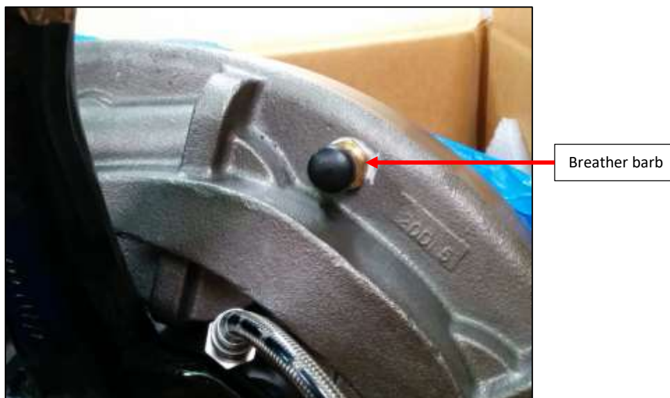
Figure 25: Breather barb on inner housing.
