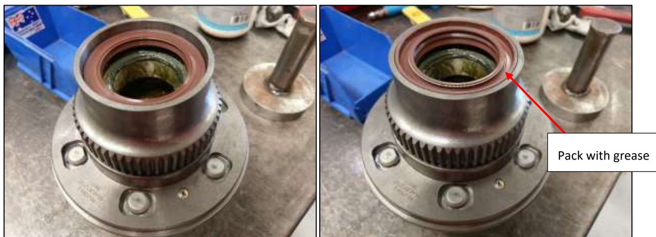
Figure 47: First shaft seal in (left) Both shaft seals in (right)
