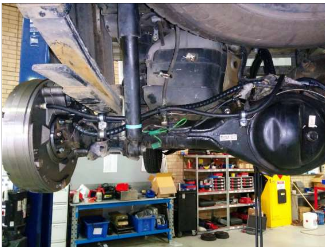
Figure 28: Brake lines routed to rear LH brake unit (facing front of vehicle).
