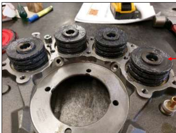
Figure 52: Lubricated springs on the pistons
