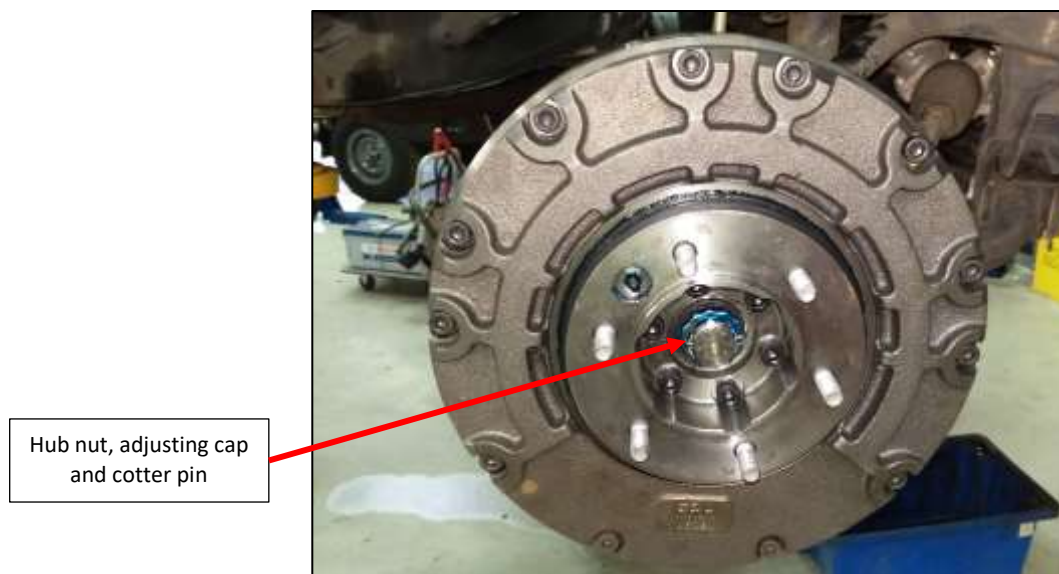
Figure 20: Install hub nut and adjusting cap.
