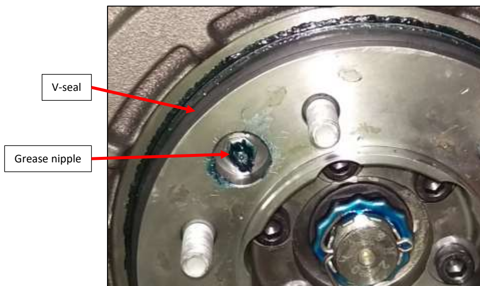
Figure 23: Grease V-seal cavity.
