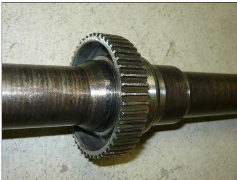
Figure 4: Press ABS pulse wheel up to circlip.
