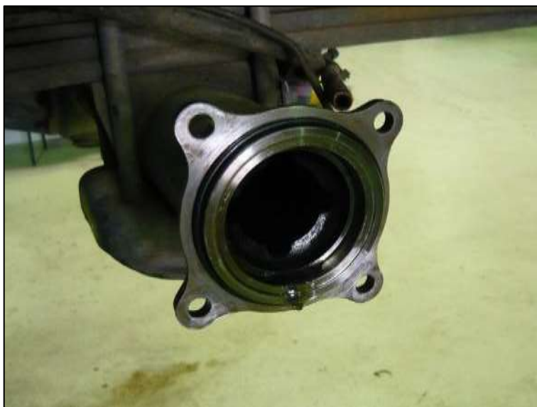
Figure 2: Fit new O-ring seal to axle flange.
