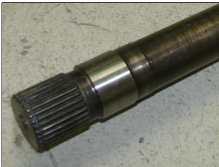
Figure 7: Fit O-ring to groove on axle shaft.
