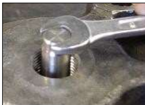
Fig 3: Pad wear indicator plunger.
