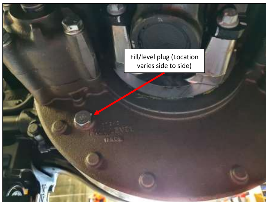
Fig 8: Failsafe Emergency brake fill/level plug (HV19 shown).
