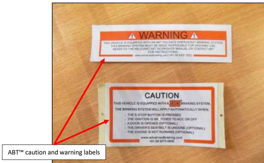
Figure 19: Failsafe Emergency labels.
