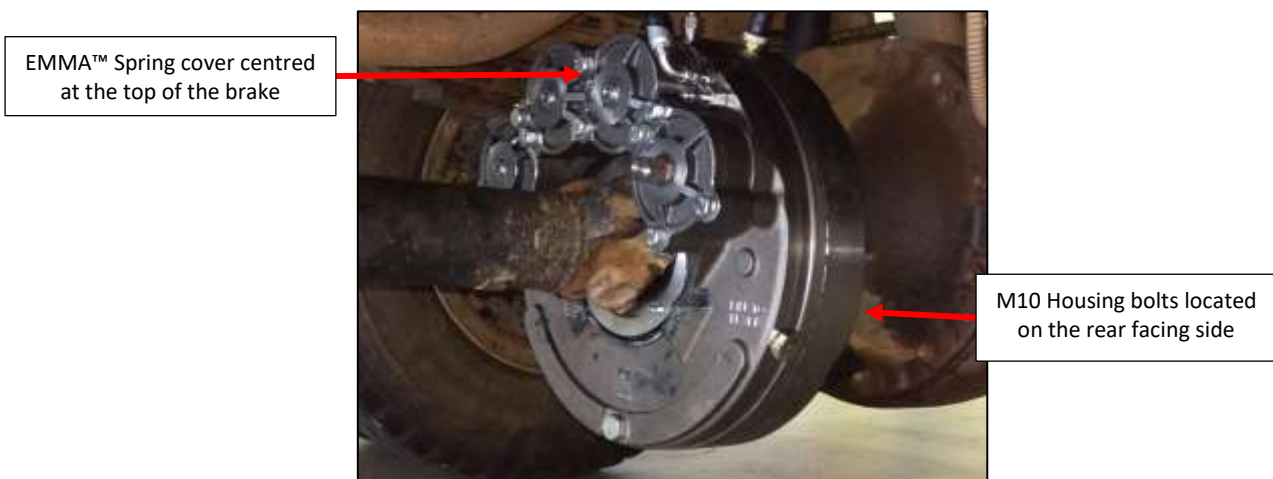
Figure 3: Brake mounted in position on the forward side of the rear diff centre.
