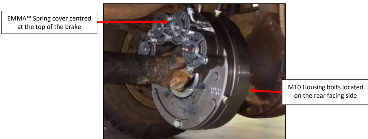
Figure 3: Brake mounted in position on the forward side of the rear diff centre.
