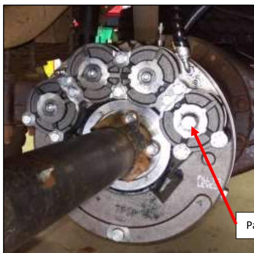
Figure 18: Brake assembly attached to rear diff centre.
