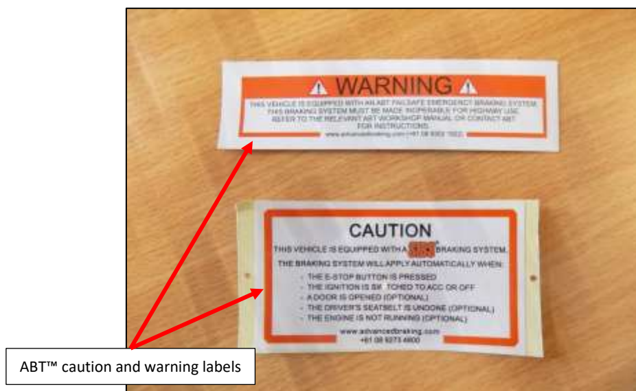
Figure 19: Failsafe Emergency labels.
