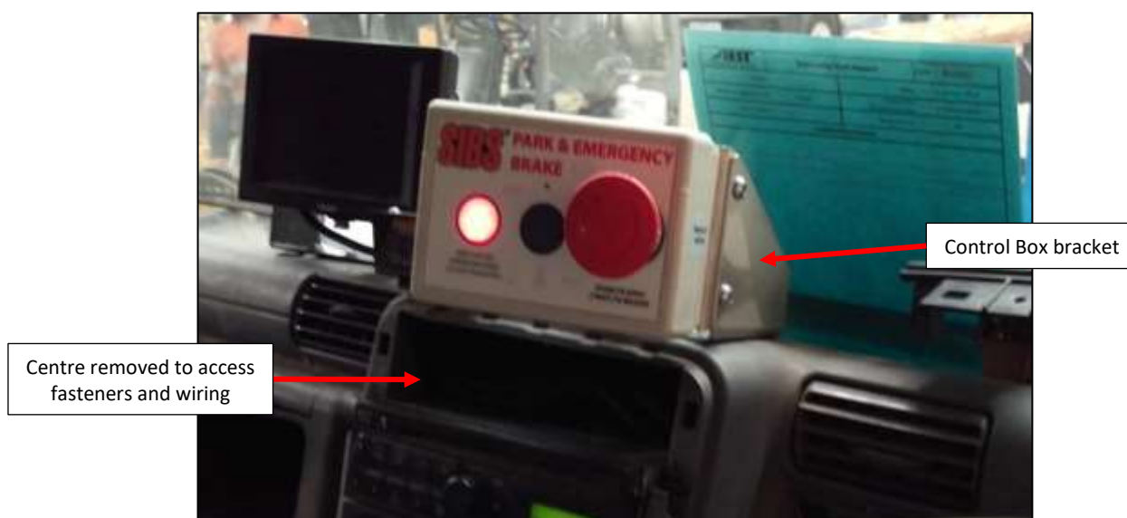
Figure 10: ABT™ Failsafe Emergency brake control unit mounted on dash.
