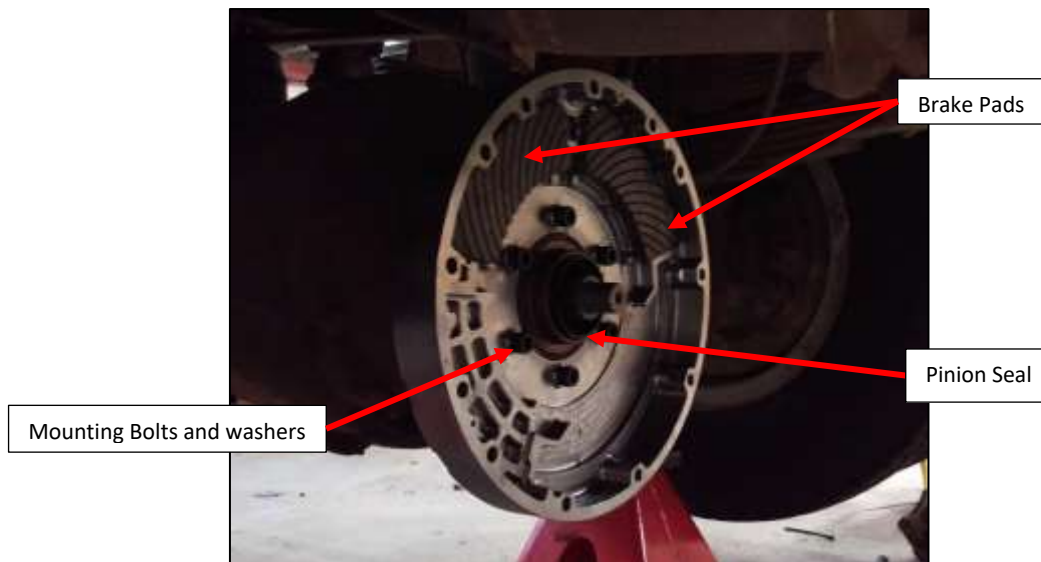
Figure 1: Diff centre with inner housing attached.
