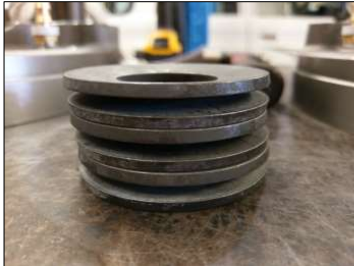
Figure 25: Disc springs installed on Failsafe Emergency brake piston.
