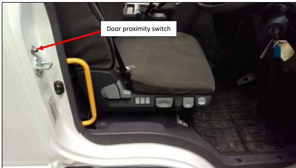
Figure 19: Door proximity sensor.
