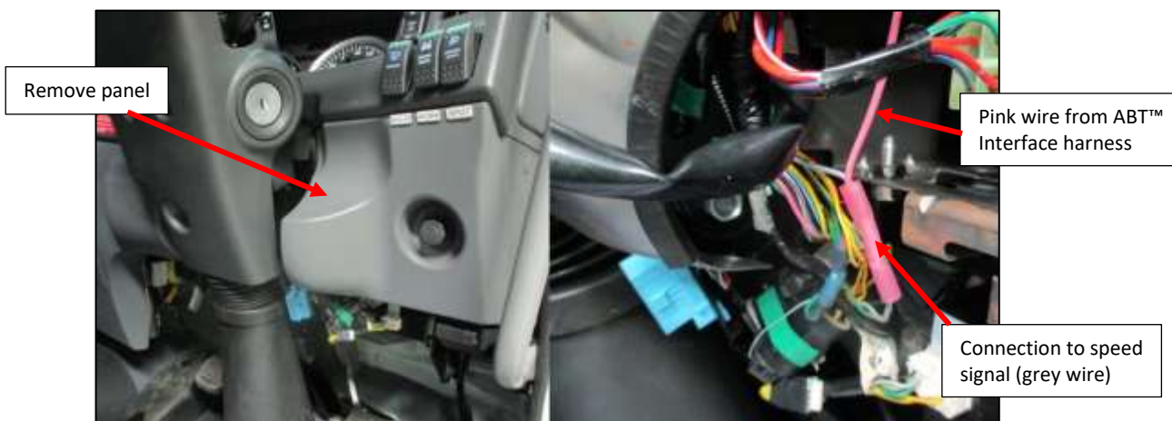
Figure 16: Connection for speed signal next to steering column.
