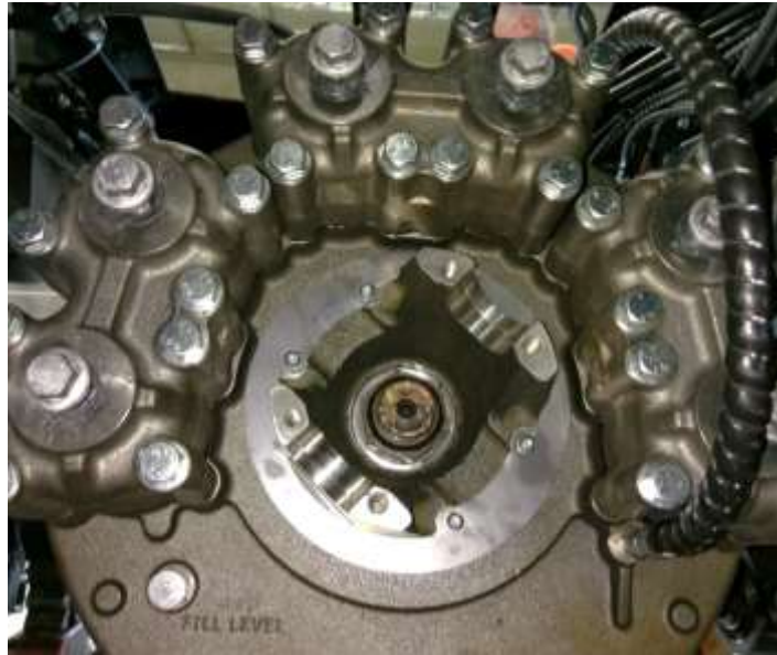
Figure 7: Assembled brake with the yoke
