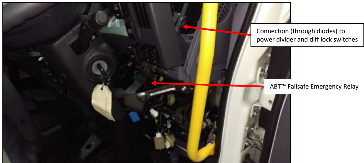
Figure 17: Connection for interlocks next to steering column.
