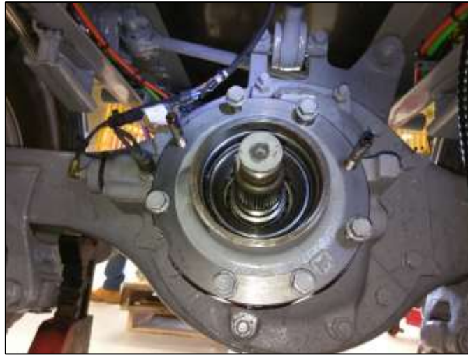
Figure 3: partially removed bearing carrier
