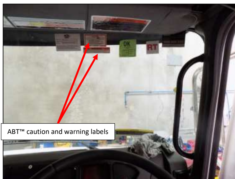
Figure 26: Failsafe Emergency labels on windshield.
