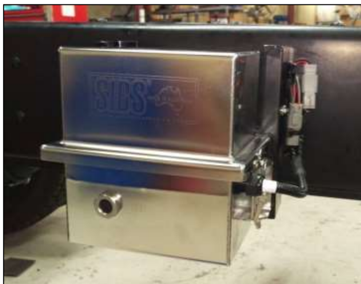
Figure 10: ABT™ Failsafe Emergency brake pump enclosure.
