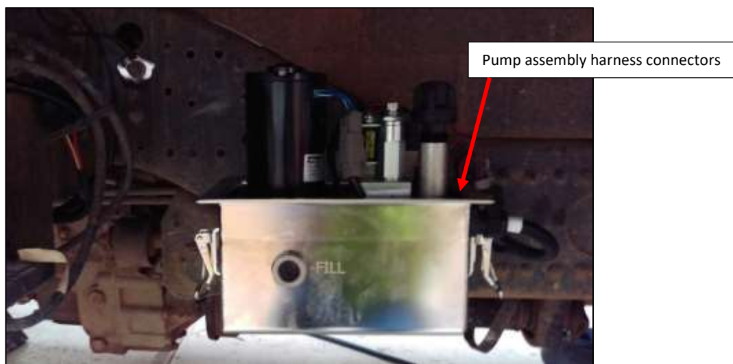
Figure 26: Pump harness connection.
