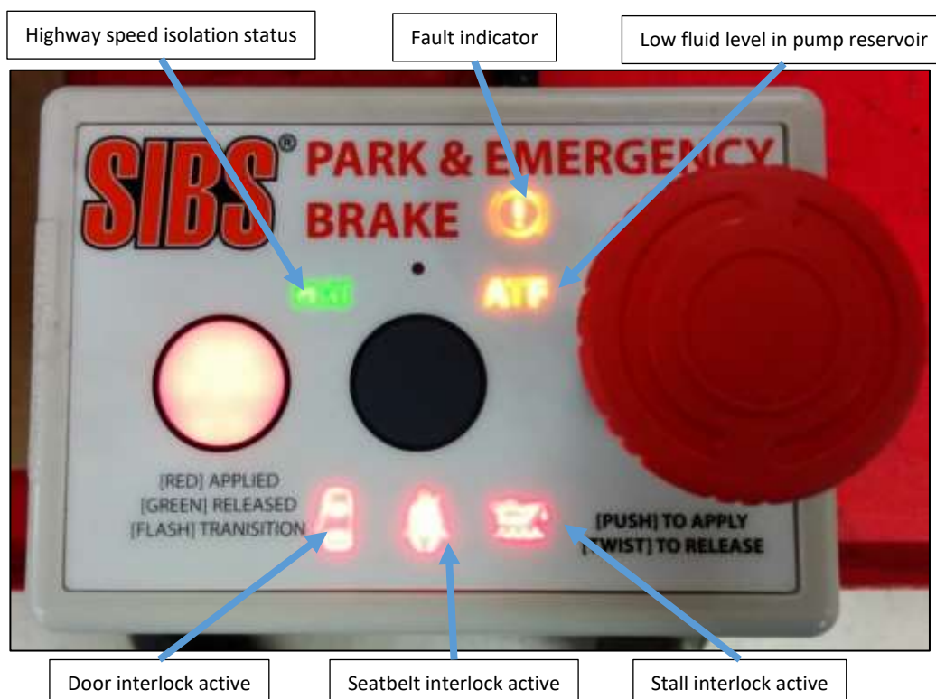
Figure 29: ABT™ Failsafe Emergency control unit warning lights
