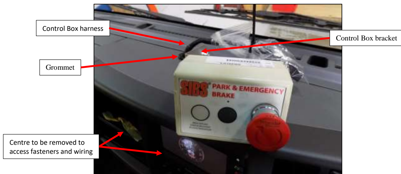
Figure 19: ABT™ Failsafe Emergency control unit mounted on dash.
