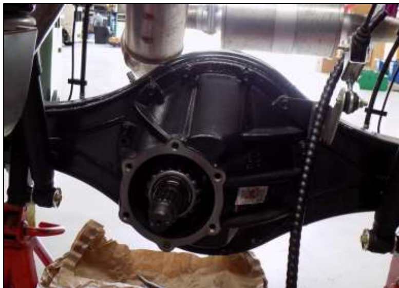
Figure 2: Rear differential carrier with bearing cage removed.
