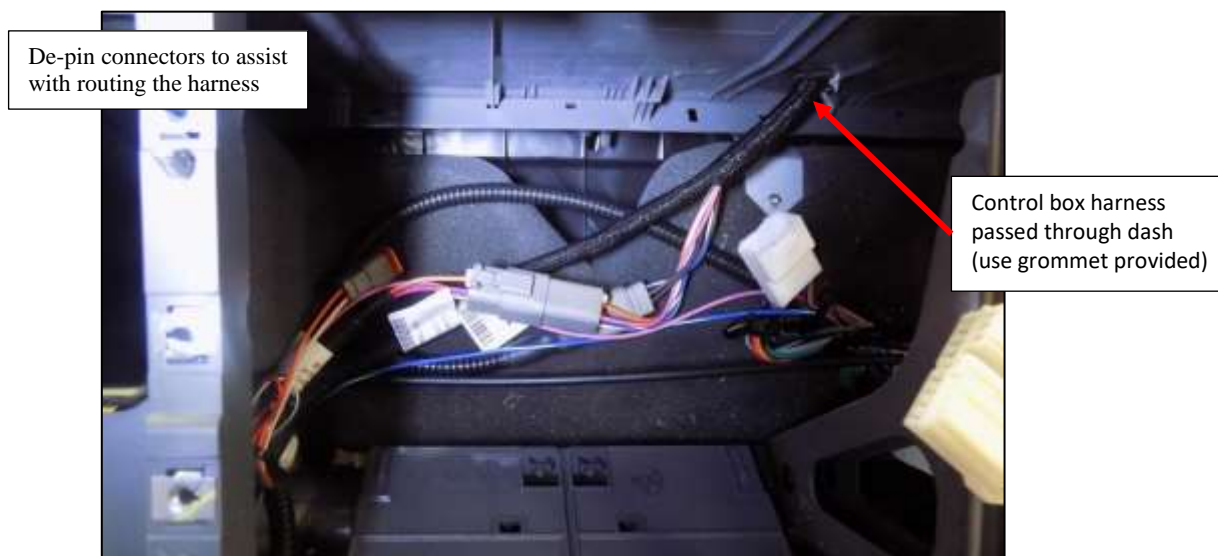
Figure 22: Control unit wiring.
