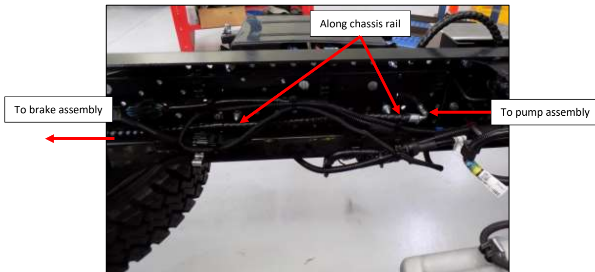
Figure 17: Hydraulic hose routing to brake.
