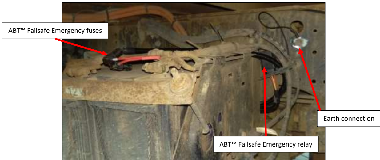
Figure 25: Battery power harness.
