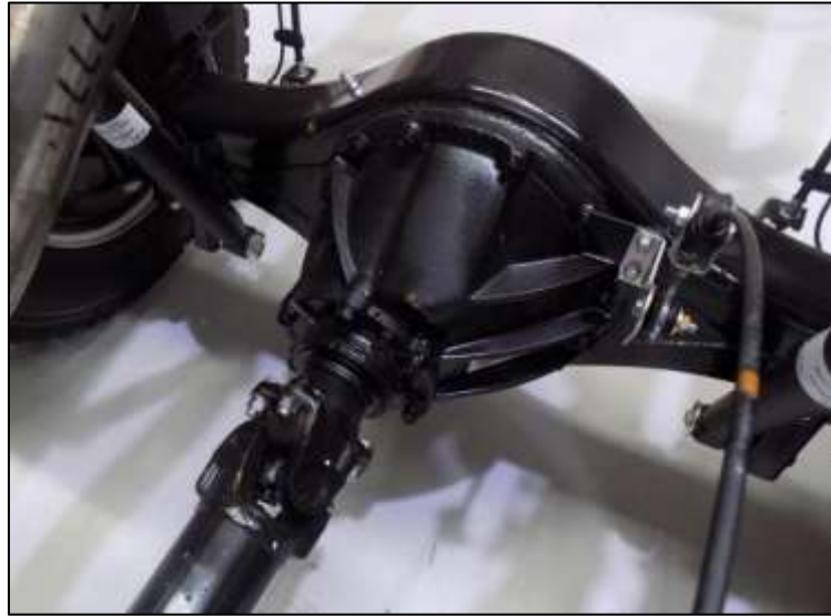
Figure 1: Rear differential carrier.
