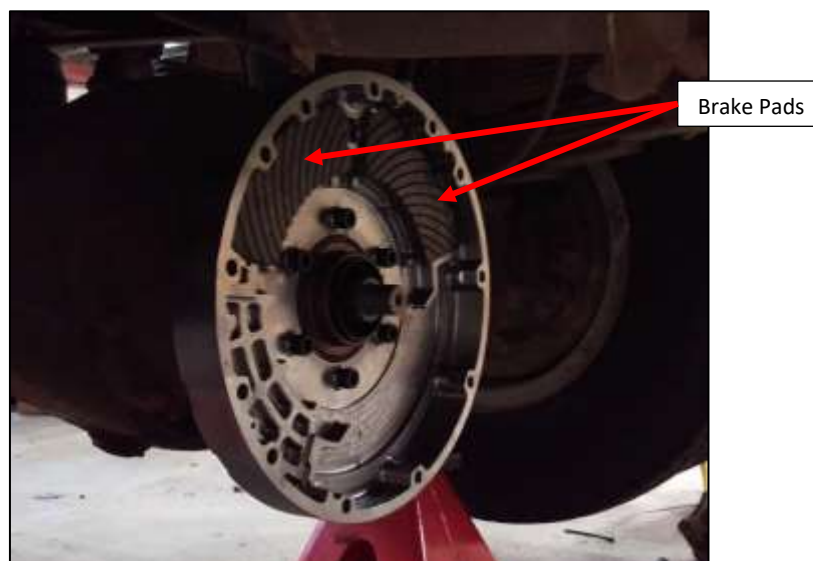
Figure 5: Inner housing with brake pads.
