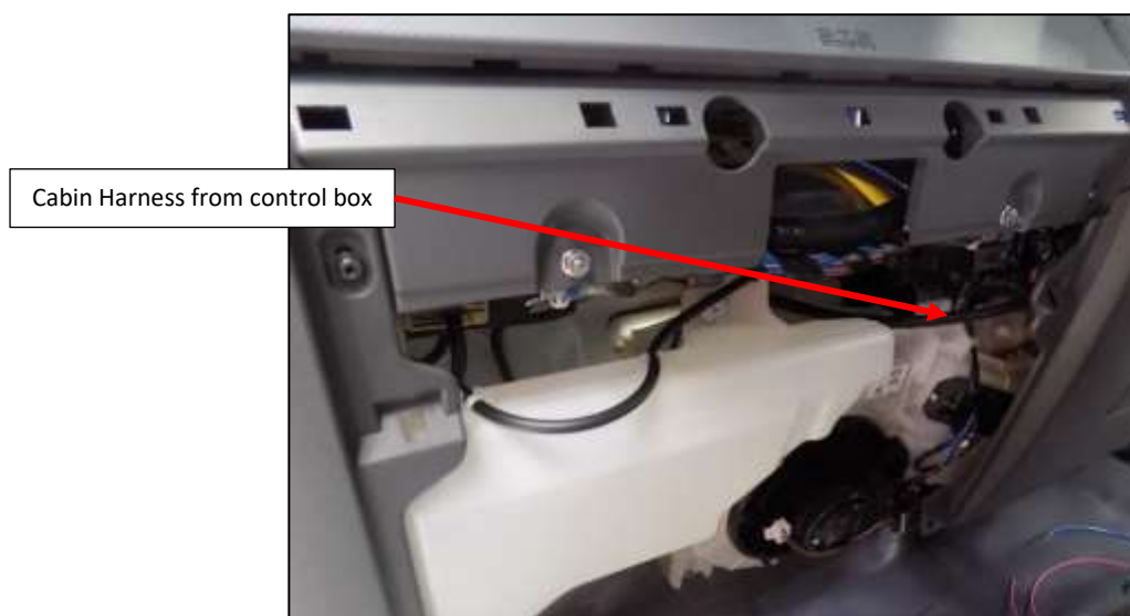
Figure 23: Cabin harness routing.
