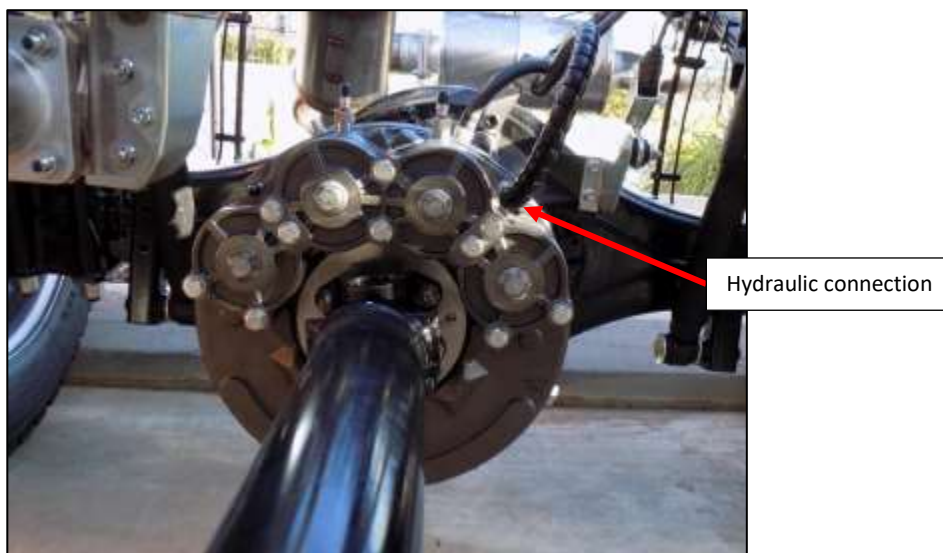
Figure 18: Hydraulic connection to brake.
