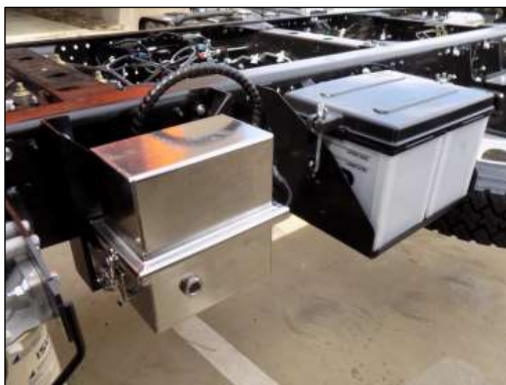
Figure 15: ABT™ Failsafe Emergency pump enclosure.
