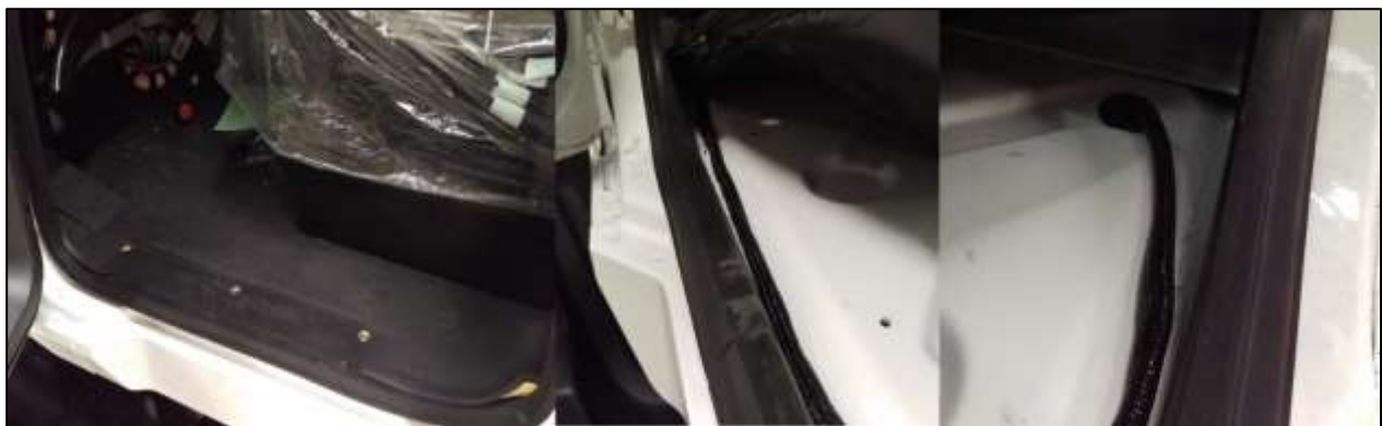
Figure 16: Cabin harness routing along floor of cab.
