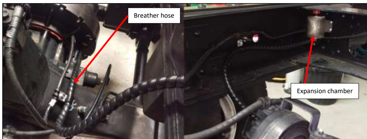
Figure 7: Brake breather hose and expansion chamber.
