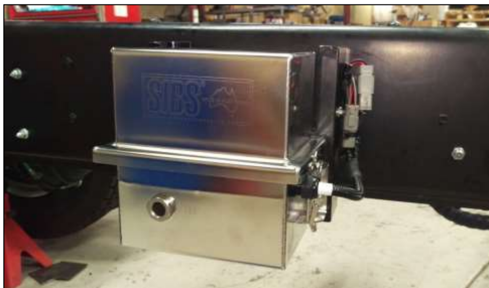
Figure 9: ABT™ Failsafe Emergency brake pump enclosure.
