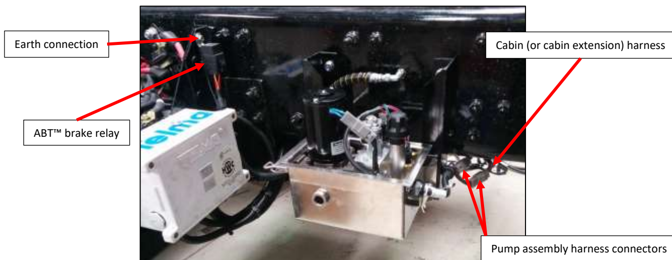
Figure 22: Pump harness connection.
