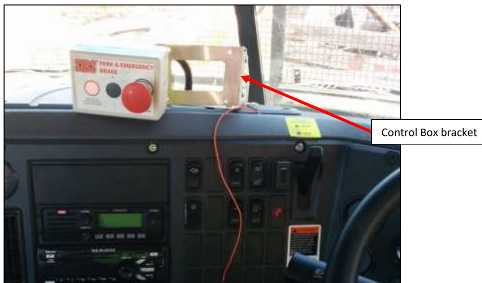
Figure 13: ABT™ Failsafe Emergency brake control unit mounted on dash.
