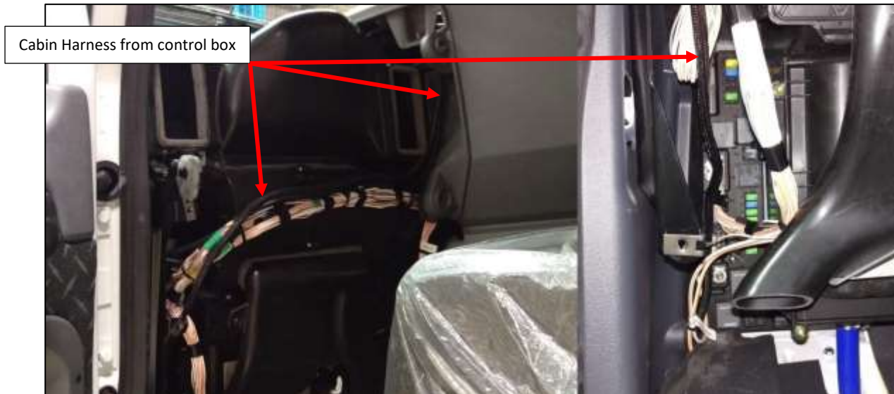
Figure 15: Cabin harness routing.
