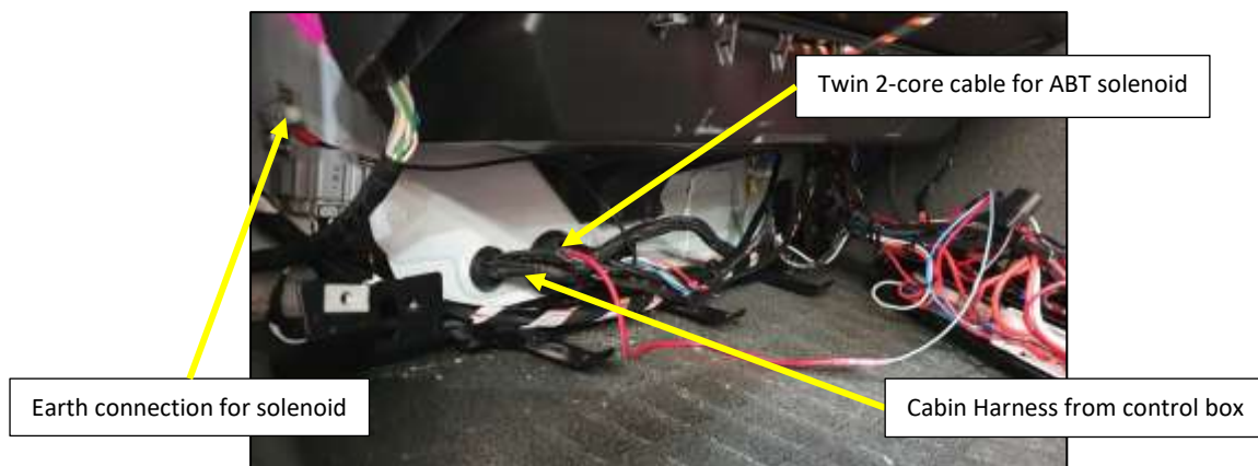
Figure 21: Connection for interface cables back of fuse board.
