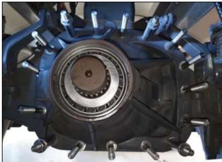
Figure 4: Outer housing, yoke and rotor assembly.
