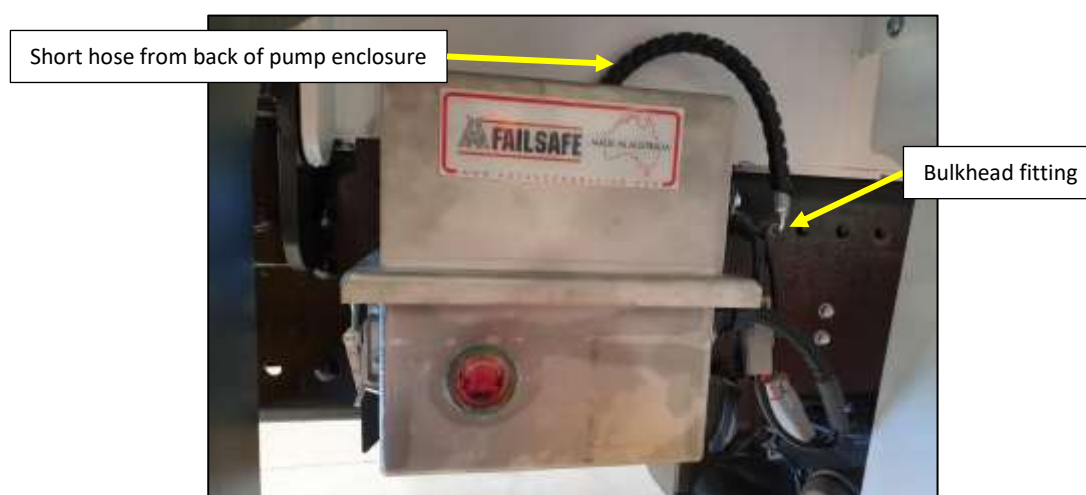
Figure 12: ABT™ Failsafe Emergency brake pump enclosure and hydraulic connections.
