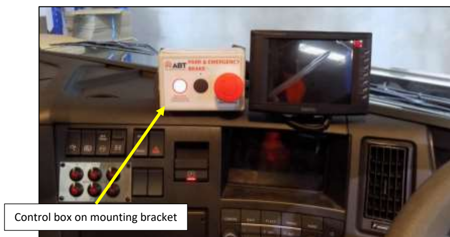
Figure 15: ABT™ Failsafe Emergency control unit mounted on dash.
