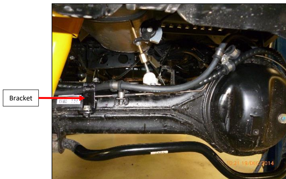
Fig. 51 Brake lines routed on to LH brake unit (facing front of vehicle).
