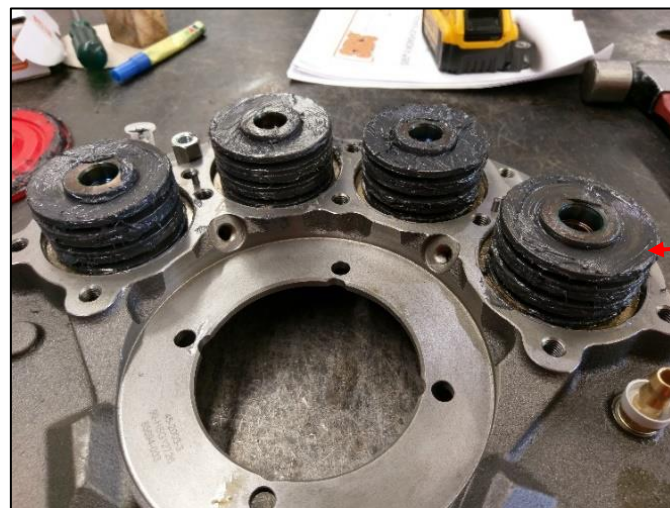
Fig. 10 Lubricated springs on the pistons
