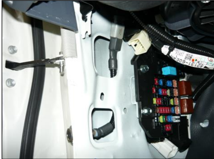
Fig. 10 Secure proximity switch with locknuts and route harness.
